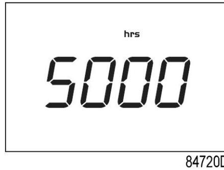
In the example shown, the screen shows the unit used <hrs> and the value <5000>: the controller module has been in service during 5000 hours.
