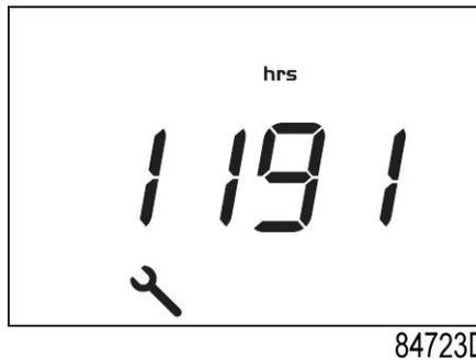
This screen shows the unit used (<hrs> or <x1000 hrs>) and the value. In the example shown, the compressor has run 1191 hours since the previous service.
