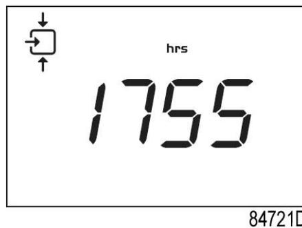
The screen shows the unit used <hrs> (or <x1000 hrs>) and the value <1755>: the compressor has been running loaded during 1755 hours.
