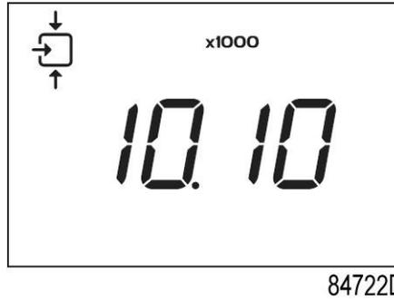
This screen shows the number of loading actions (x1 or - if <x1000> lights up - x1000). In the above example, the number of unload to load actions is 10100.
