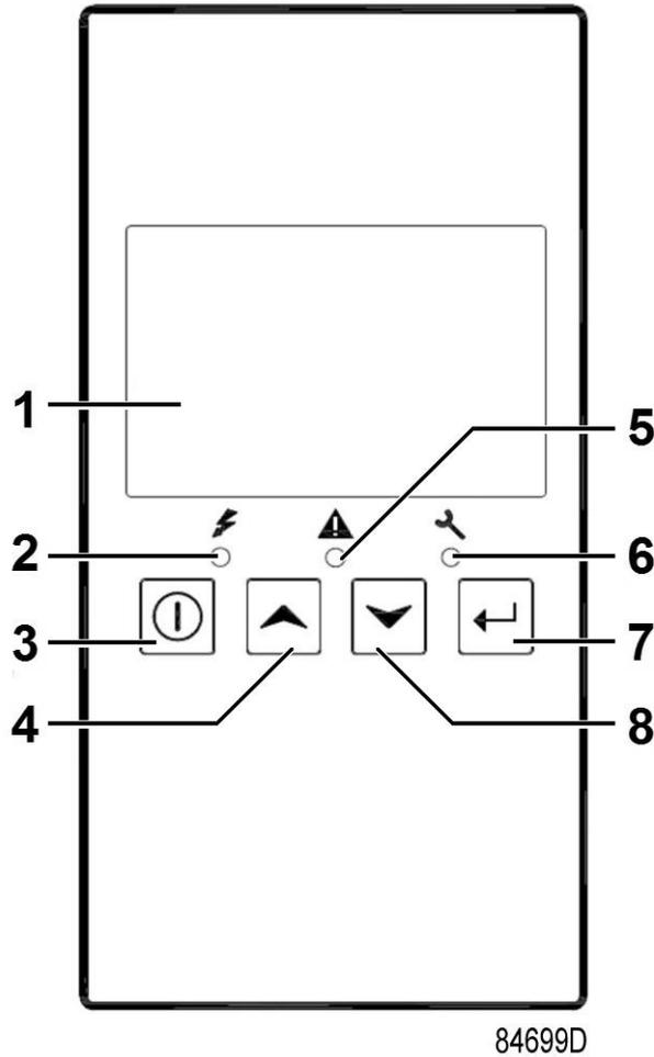
It remains possible to check the actual status of other parameters by pressing the enter button (7) for 3 seconds. Press button (3) to stop the compressor and wait until the compressor has stopped. The warning message will disappear as soon as the warning condition disappears.
