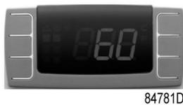
6. Select desired service interval using the UP or DOWN button.
