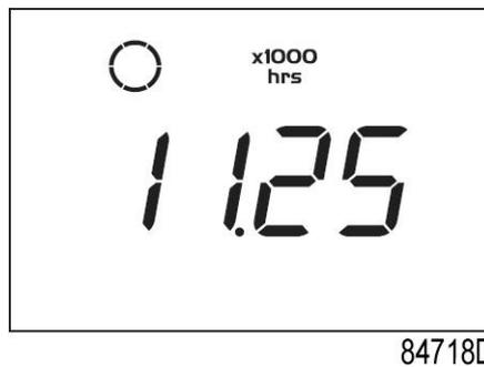
The screen shows the unit used <x1000 hrs> and the value <11.25>: the running hours of the compressor are 11250 hours.
