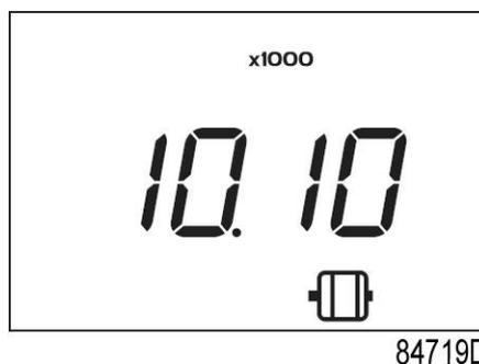
This screen shows the number of motor starts (x1 or - if <x1000> lights up - x1000). In the above example, the number of motor starts is 10100.
