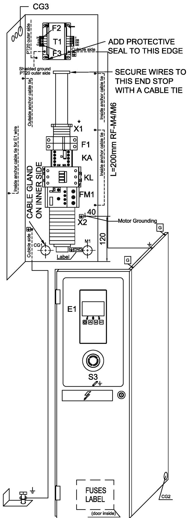
**35 - Cubicle components QGS 15 - 208-230-460V/60Hz - UL-cUL (11/10/2016 - 11/12/2023)**
