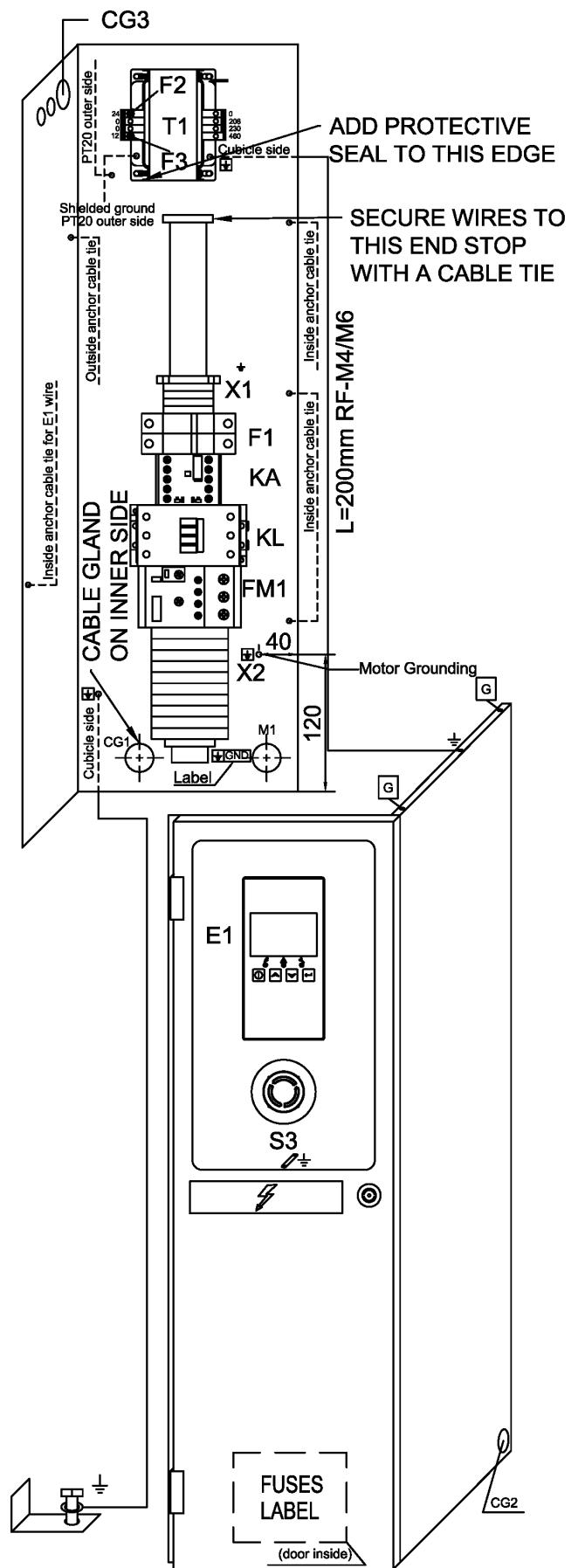
**33 - Cubicle components QGS 10 - 208-230-460V/60Hz - UL-cUL (11/10/2016 - 11/12/2023)**
