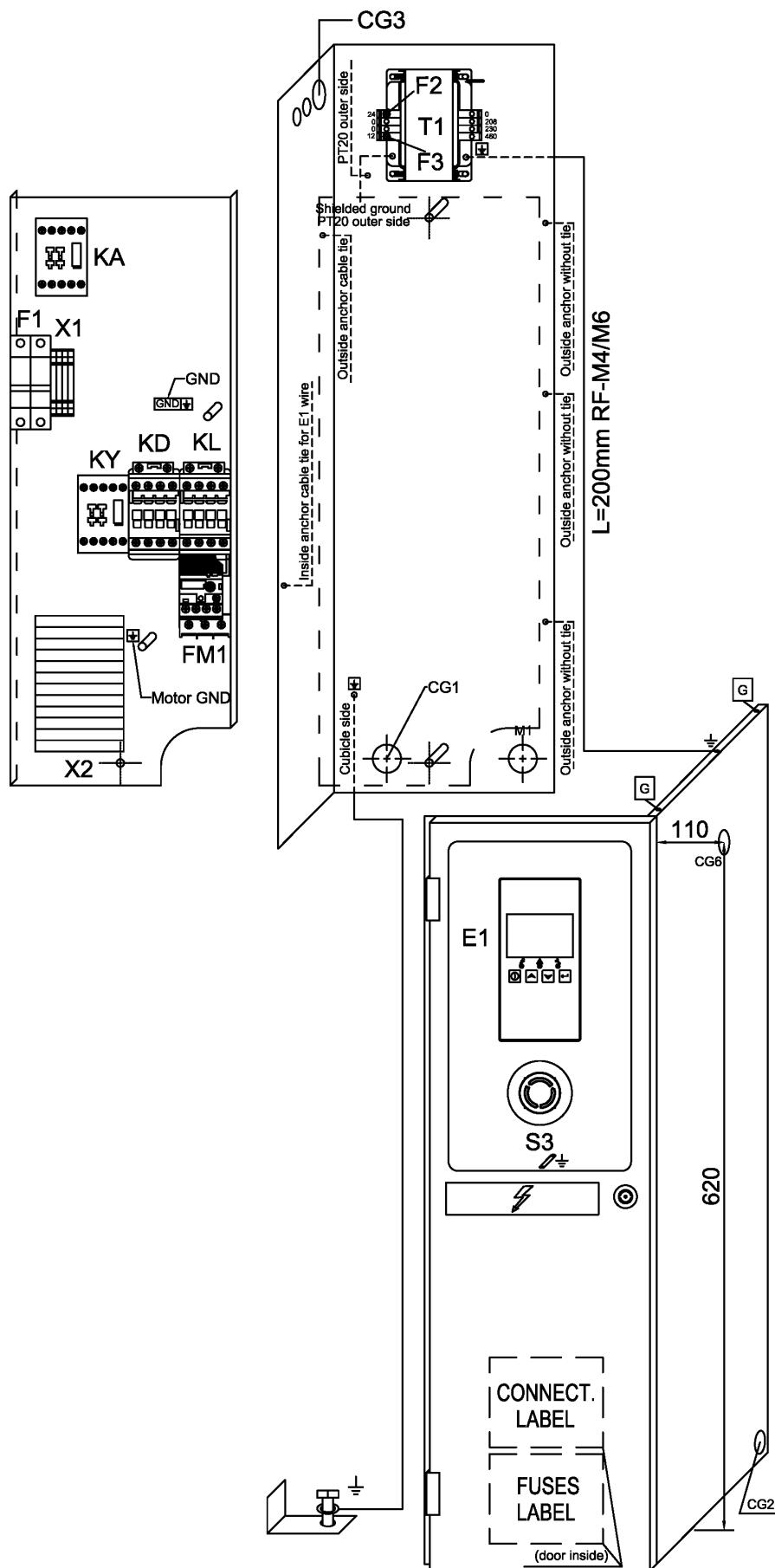
**37 - Cubicle components QGS 20S - 208-230-460V/60Hz - UL-cUL (11/10/2016 - 11/12/2023)**
